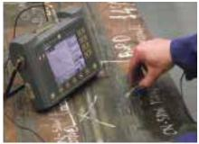
Manual ultrasonic testing of a plate
