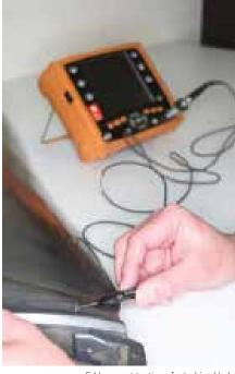
Eddycurrent testing of a turbine blade
