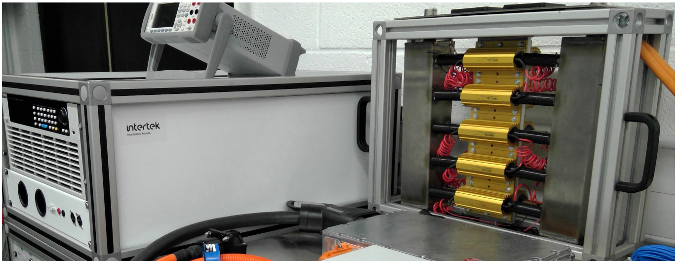
HV junction box undergoing dynamic load carrying test
