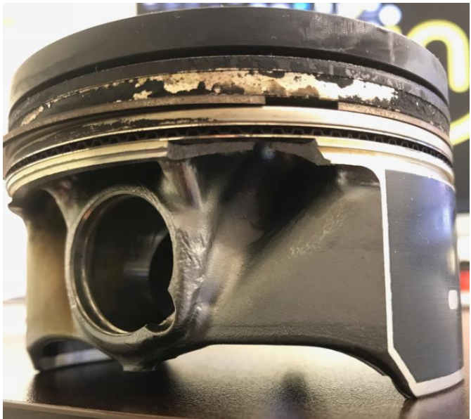
Piston damage due to preignition events
